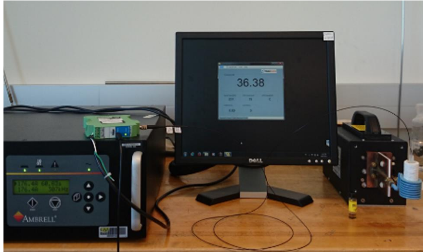
Figure 2.2 Magnetic hyperthermia system employed. Generator on the left and radio frequency amplifier on the right.
